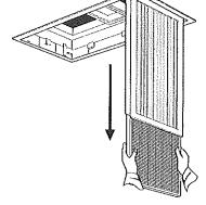
7. If a fresh air filter is fitted turn clips through 90° and remove filter.
