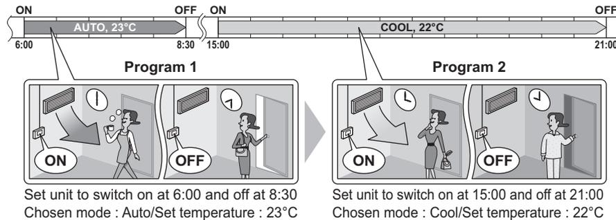
**Case 2** The MULTI 7 DAY TIMER can be programmed to start & stop the air conditioning unit twice a day, 7 day a week. Individual modes, temperatures, zones & sensor position can also be set within each time frame.
