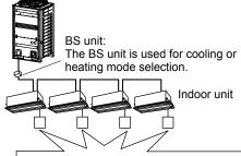
A single BS unit is connected to a number of indoor units.
