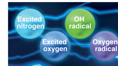
The electrons collide and combine with nitrogen and oxygen in the air to form four kinds of elements with powerful oxidative decomposition capabilities.
