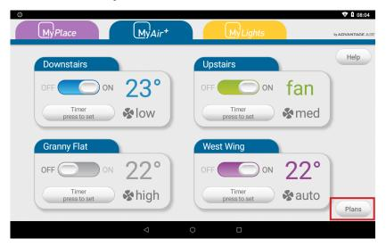
MyAir+ Plans apply to all of your air-con units, this means that the "captured" snapshot for the plan will include the state of all air-cons in your system as well as all the zone settings for each of the air-cons.
