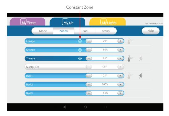
In this example these two zones may open automatically to relieve excess air pressure when needed.
