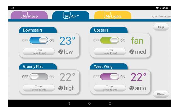
When the MyPlace app is started the MyAir+ tab will display the home screen as shown above. Each icon set above represents a separate air-con, pressing on the top left of an icon will open that air-con unit. Each air-con unit can be controlled the same way as any MyAir system.
