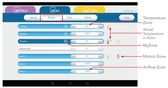
Pressing a Zone name toggles that Zone between ON and OFF. Zones are OFF when they are in grey colour.
