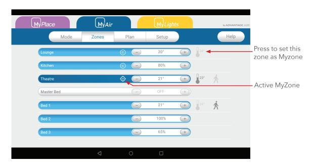
This feature can be particularly important when you have an unusually high requirement for air conditioning in a particular area. For example, a group of people watching a movie in Theatre room with all the electronic A/V equipment turned on will have a larger requirement for air conditioning than in other rooms in the house. Setting the Theatre as MyZone will ensure that the system continues running until the temperature set-point for that room is achieved.
